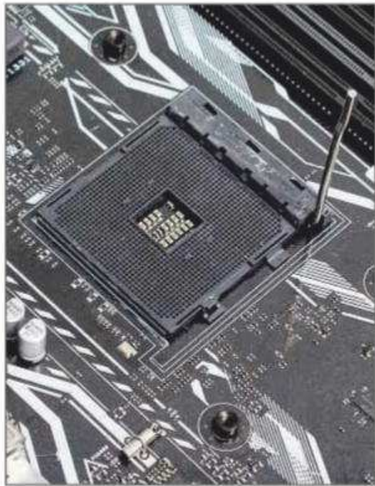
To install a CPU on an AMD AM4 system, you first need to lift the handle next to the socket
