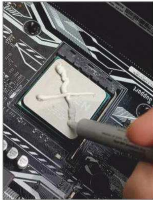
Apply the thermal paste to your chip in a cross shape
